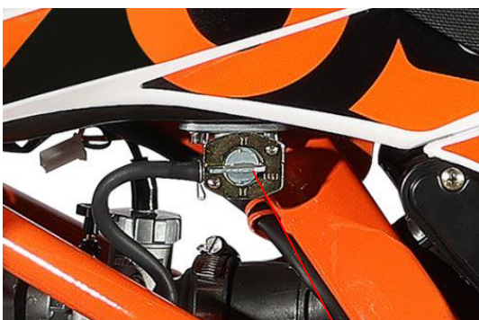
Fuel tank switch
