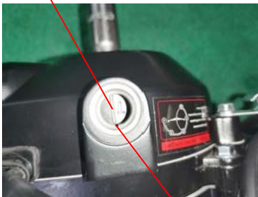
Engine left front cover timing mark
