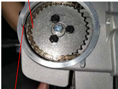
Timing mark of cylinder head
