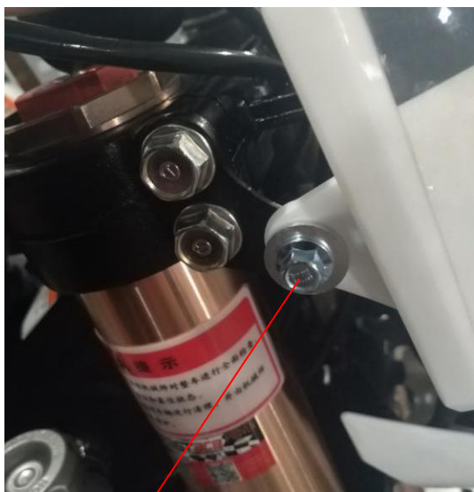
Fixing Bolts on Upper Bracket
