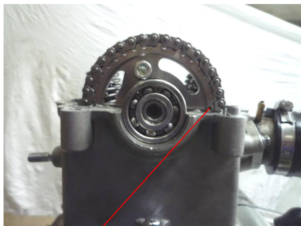
Timing mark for timing driven sprocket
