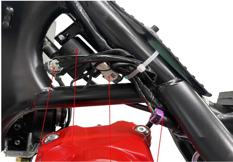
1、 Fan connectors 2、 High voltage package 3、 Ignition coil and spark plug Connectors 4、 Rectifier regulator connector
