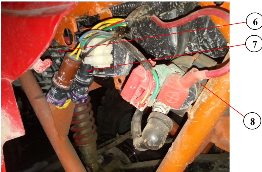
6、 Voltage regulator rectifier 7, charging connector 8, relay
