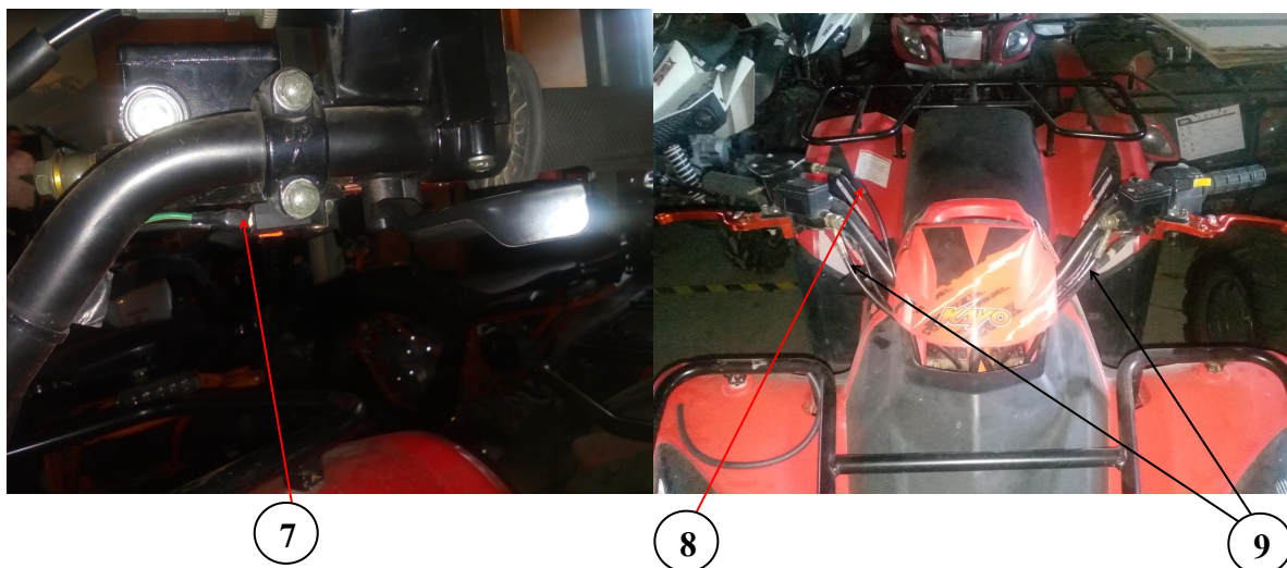
7, brake sensor (left one and right one) 8, throttle line 9, brake hose
